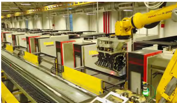
Mercury's new array of Mazak automated conveyances and machining robots move engine blocks through the process.
