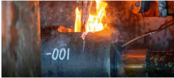
All of the aluminum in the patented alloy that Mercury uses in its castings is recycled. Here, molten alloy goes into the pouring hole of the die-cast machine's hydraulic cylinder. The machine will inject the material into a die mold under as much as 4,500 tons of pressure.
