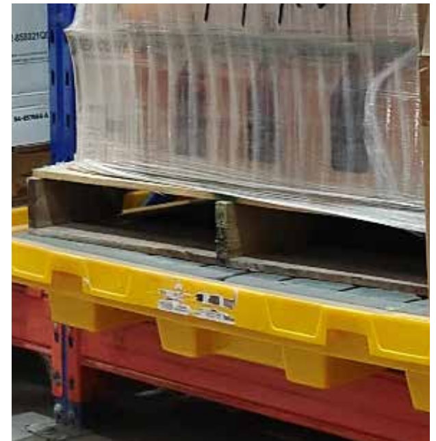
In Suzhou, China, Mercury uses plastic pallet bases, cofferdams and leak-proof flooring to protect the environment from oils, chemicals and other industrial fluids.
